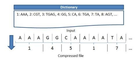
Figure 2: Example for dictionary-based algorithms
