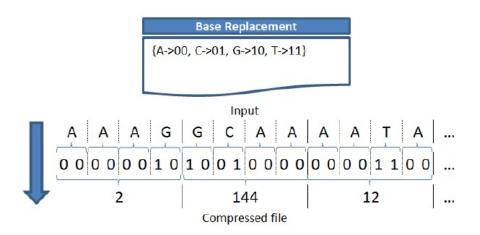
Figure 1: Example for naive bit encoding
